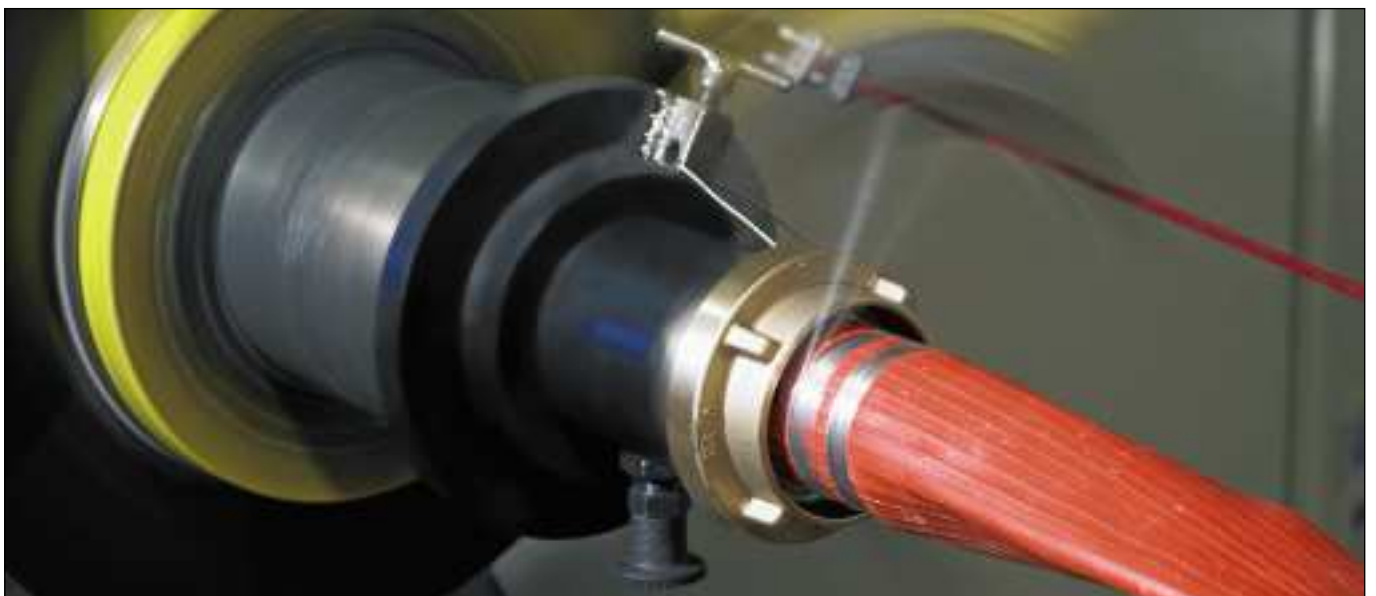
Assembly of Storz coupling to Guardman hose
